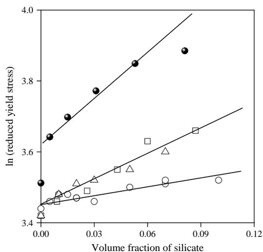
Fig. 5. Reduced tensile yield stress of the composites shown in Fig. 4 plotted against filler content in linear form. Symbols are the same as in Fig. 4.
