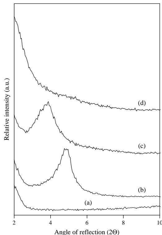
Fig. 3. XRD pattern of PP/clay composites and their components; disappearance of the silicate reflection upon the introduction of MAPP. (a) PP+20 v/v % MAPP blend, (b) OMMT (c) PP+2 v/v% OMMT, (d) PP+2 v/v% OMMT+20 v/v% MAPP.
