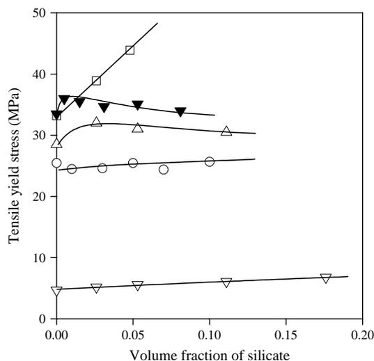
Fig. 6. Tensile yield stress of several PP/OMMT/MAPP composites plotted as a function of silicate content. See the details in Table 1. Symbols: (□) Reichert [19] (15), (▽) Chen [73] (28), (○) this paper (31), (▼) Svoboda [71] (24), (△) Manias [12] (26).
