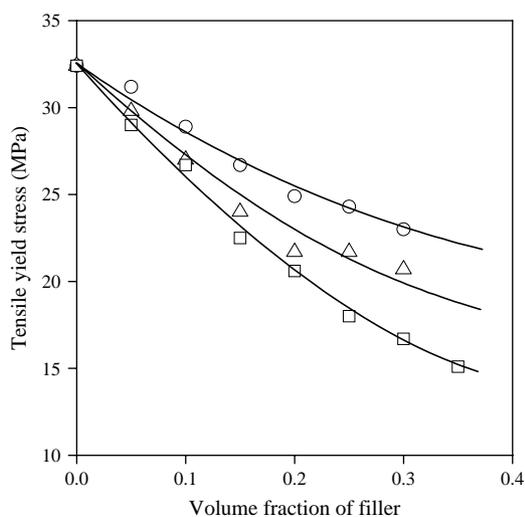
Fig. 1. Effect of particle size and filler content on the tensile yield stress of PP/CaCO<sub>3</sub> composites. Specific surface area ( $A_T$ ): (○) 5.0, (△) 3.3, (□) 0.5 m<sup>2</sup>/g.
