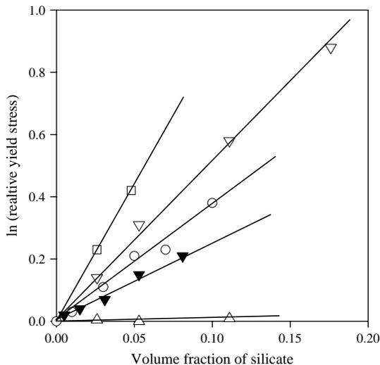
Fig. 7. Relative tensile yield stress of the composites shown in Fig. 6 plotted as function of silicate content in the linear form of Eq. (4). Symbols are the same as in Fig. 6.
