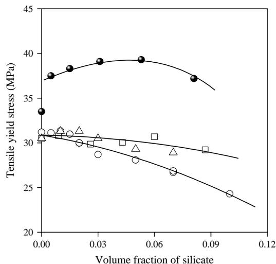
Fig. 4. Effect of silicate content on the tensile yield stress of various PP/clay composites. See the details in Table 1. Symbols: (□) PP/NaMMT (34), (Δ) PP/OMMT (37), (○) PP/OMMT/MAPP (41), (●) PP/OMMT/MAPP [71] (22).
