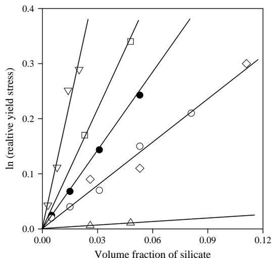
Fig. 8. Evaluation of yield stresses according to Eq. (4). Results taken from the literature in the entire range of reinforcing effects. Symbols: ( $\nabla$ ) Liu [74] (20), ( $\square$ ) Reichert [19] (13), ( $\bullet$ ) Svoboda [71] (22), ( $\circ$ ) Svoboda [71] (24), ( $\diamond$ ) Kaempfer [47] (17), ( $\triangle$ ) Reichert [19] (5). See the details in Table 1.
