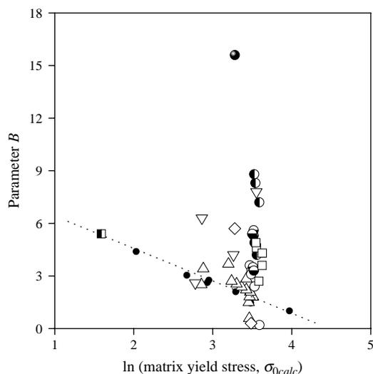
Fig. 10. Estimation of the reinforcing effect of layered silicates in PP composites (Eq. (6)). Symbols: (○) Reichert [19] (1–5), (●) Reichert [19] (6–10), (●) Reichert [19] (11–15), (□) Svoboda [71] (21–25), (△) this paper (29–41), (●) Liu [74] (20), (▽) Walter, Kaempfer [45,47] (16–19), (◇) Manias [12] (26–27), (■) Chen [73] (28), (●) CaCO<sub>3</sub> reference line (dashed) shows the effect of changing matrix properties.
