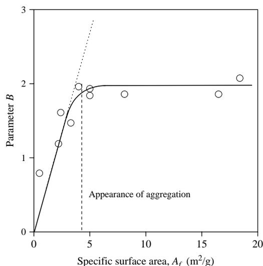
Fig. 11. Correlation between parameter  $B$  and the specific surface area of the filler ( $A_f$ ) for PP/CaCO<sub>3</sub> composites.
