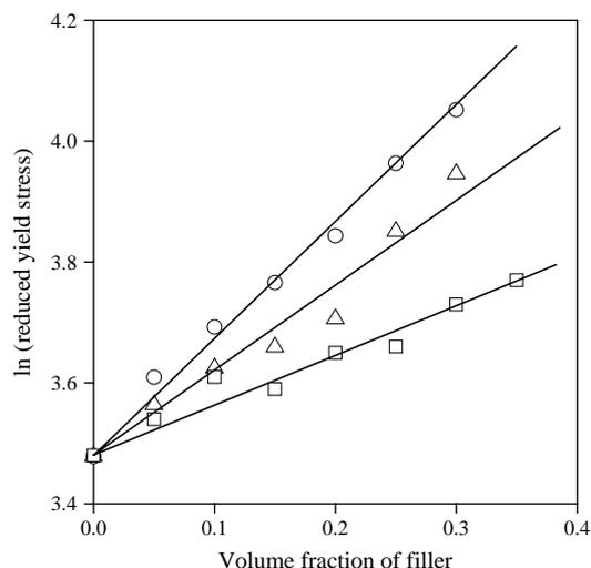
Fig. 2. Linear representation of reduced yield stress for the composites shown in Fig. 1 supporting the validity of the model (Eqs. (1)–(3)). Symbols are the same as in Fig. 1.
