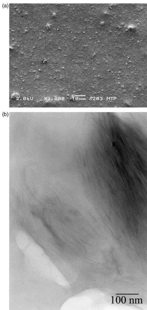
Fig. 12. Structure of a PP/OMMT/MAPP composite containing 20 vol% MAPP and 2 vol% silicate, (a) SEM, (b) TEM.
