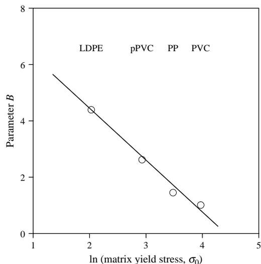
Fig. 9. Effect of matrix yield stress on the relative load bearing capacity of the filler (parameter  $B$ ) [39].
